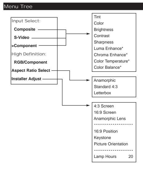
The menu tree above is an overall glance at the menu system in the DR-300c. This menu is shown with the installation mode enabled.
